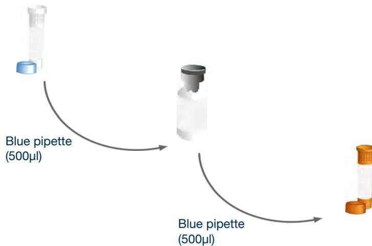
Use the blue pipette to transfer 500µl of the oasis mastermix resuspension buffer into the tube of lyophilised oasis mastermix and mix well by inversion. Then transfer all of that mastermix into the brown tube labelled A.hydrophila primers/probe.
