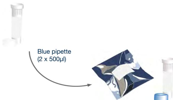
Use the blue pipette to transfer 1000 $\mu$ l (2 x 500 $\mu$ l) of water into the Internal Extraction Control DNA tube. Cap and shake tube to mix.
