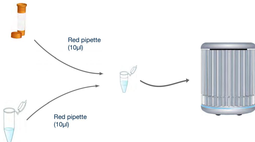
For each sample you wish to analyse, use the red pipette to combine 10 $\mu$ l of your *A.hydrophila* reaction mix with 10 $\mu$ l of your DNA sample in the reaction tubes provided. Always change pipette tips between samples.
