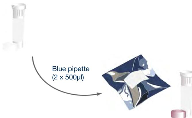
Use the blue pipette to transfer 1000µl (2 x 500µl) of water into the positive control template tube. Cap and shake tube to mix.
